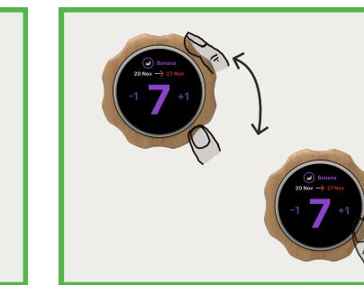
7 The screen displays the average shelf life of each food item in the database, and the date can be adjusted autonomously by rotating it and then pressing to confirm it
